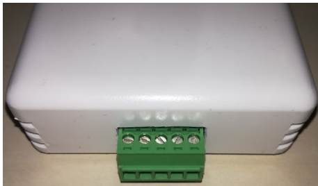
Fig. 3 Power supply and RS-485 interface connector
